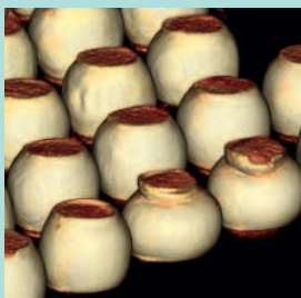
Visualization of head-on-pillow defects in 2D view and 3D view
